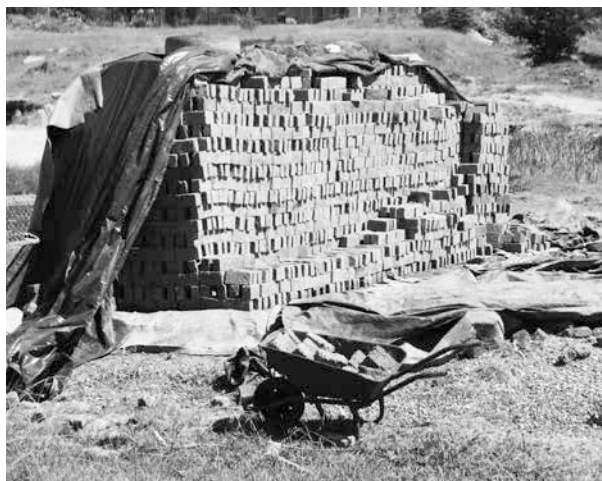
FIGURE 78 Bricks ready for burning by an informal manufacturer, Maseru East
